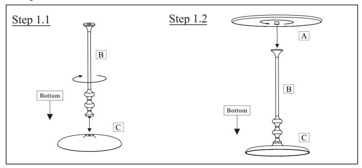
Step 1.1- Place the Base (C) on a non-marring flat surface. Align threaded end of the Stem (B) onto Base (C) as shown above in the drawing. Rotate Stem (B) in clockwise direction until secured.
